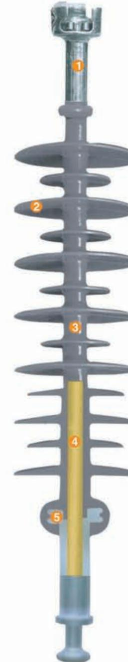
1. End Fitting: The fitting connection adopts the zinc cover protection, supersonic monitor and coaxial constant compression controlled by computer, finished with good appearance and high quality.
